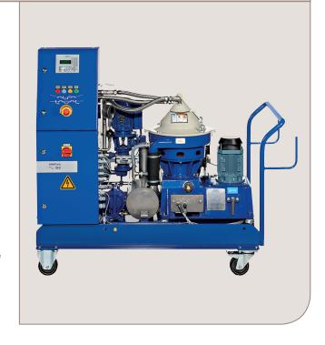
Due to their high speed, disc stack technology, and automatic discharge, Alfa Laval centrifugal separators are an extremely efficient and fast way to remove fine solid particles or liquid contaminants from different kinds of service fluids, using either a two-phase or a three-phase AlfaPure S2 module version.
