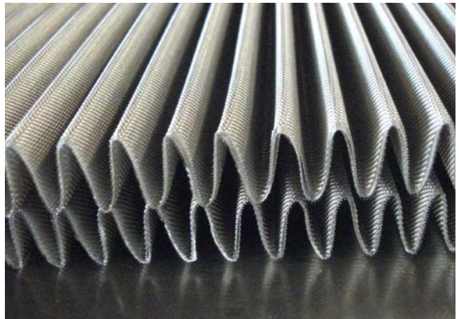
Triple layer, pleated, filter mesh: fine mesh between two support meshes.
