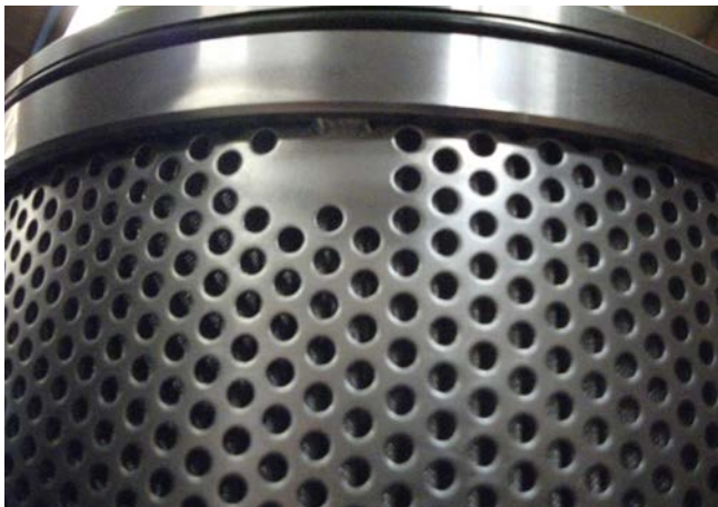
Support frame of perforated stainless steel.
