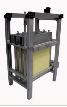
Alfa Laval Iso-Disc® cloth media filter is engineered as a continuous operating process that utilizes fixed cloth media and a dynamic, linear backflush system controlled by a PLC or relay control panel. All submerged components are corrosion resistant stainless steel or non-metallic materials.
