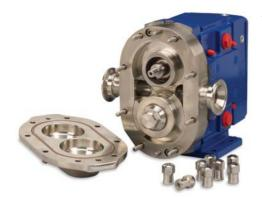
Alfa Laval rotor wings (pistons) rotate around the circumference of the channel in the pump casing. This continuously generates a partial vacuum at the suction port as the rotors unmesh, causing fluid to enter the pump. The fluid is transported around the channel by the rotor wings, and is displaced as the rotor wings re-mesh, generating pressure at the discharge port. Direction of flow is reversible.
