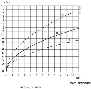
B) d = 4.6 mm Nozzles C) d = 3.9 mm
