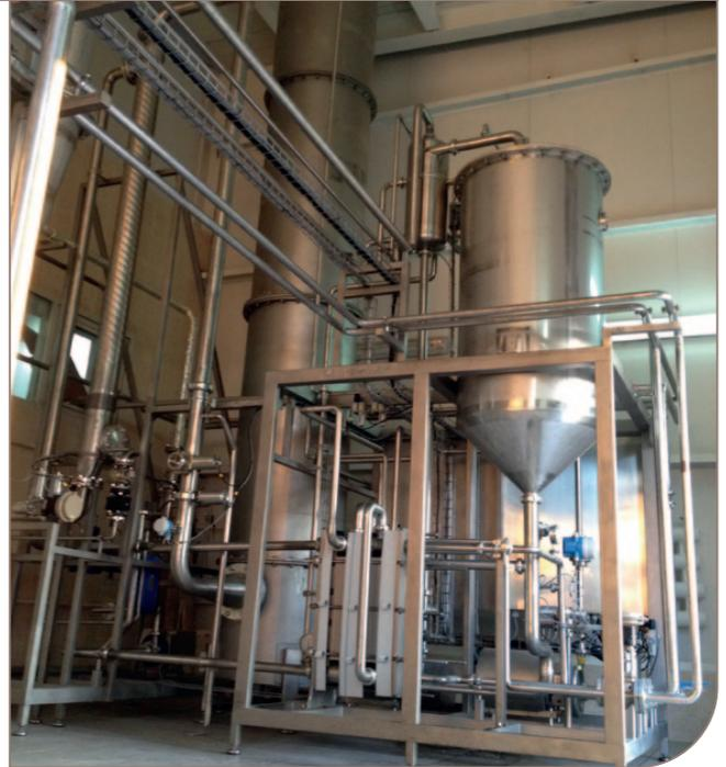
Degassing vessel and stripping column of the Alfa Laval De-alcoholization Module
