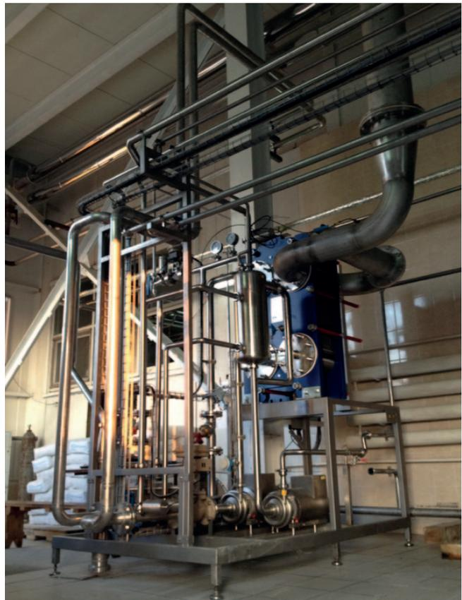
The de-alcoholization module's condensate cooling section
